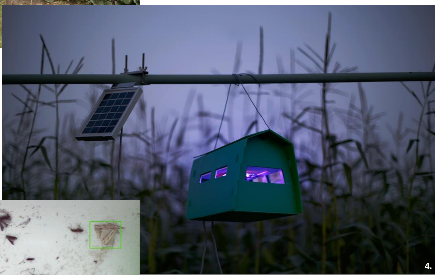
Figure 4: During activation, TrapView AURA emits near UV wavelength light. Activation and durance of emitting is managed remotely and easily. Photo: TrapView
